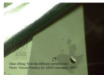
Glass Filling: Note the different surface luster. Photo: Vincent Pardieu, for AIGS Laboratory, 2002
